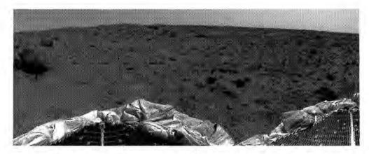
to acquire consistent lighting and shadow conditions for all areas of the panorama. At left is a lander petal and a metallic mast that is a portion of the low-gain antenna. Deflated air bags are visible at the perimeters of all three lander petals. (NASA image no. PIA00752)
