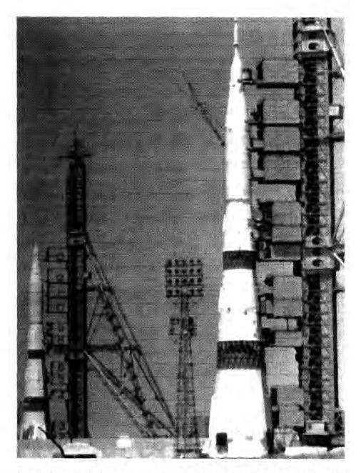
Two N1 Moon rockets appear on the pads at Tyura-Tam in early July 1969. Highly automated, the N1 was designed for the Soviet space program's human lunar missions. In the foreground is booster number 5L with a functional payload for a lunar-orbiting mission. In the background is the IMI ground-test mock-up of the N1 for rehearsing parallel launch operations. After takeoff, the rocket collapsed back onto the pad, destroying the entire pad area in a massive explosion. (NASA photo no. n1july1969)
