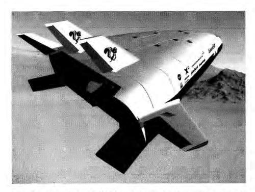
This artist's concept shows the X-33 Advanced Technology Demonstrator, a subscale prototype reusable launch vehicle (RLV), in its 1997 configuration. Named the VentureStar™, this vehicle was to have been manufactured by Lockheed Martin's "skunk works." The VentureStar™ was one of the earliest versions of the RLVs developed in an attempt to replace the aging Shuttle fleet. The X-33 program was discontinued in 2001 without flight. (NASA MSFC image no. MSFC-9711197)
