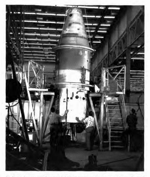
An Agena A spacecraft for an early MIDAS launch undergoes a weight test in 1960 at Lockheed's plant in Sunnyvale, California, before shipment to Cape Canaveral for launch. (Official USAF photo. Air Force Space Command, Office of History)
