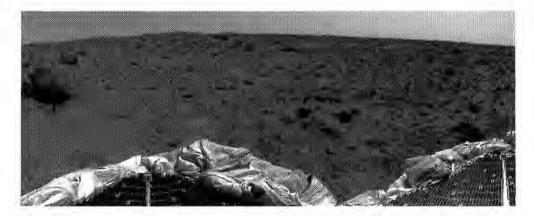
to acquire consistent lighting and shadow conditions for all areas of the panorama. At left is a lander petal and a metallic mast that is a portion of the low-gain antenna. Deflated air bags are visible at the perimeters of all three lander petals. (NASA image no. PIA00752)
