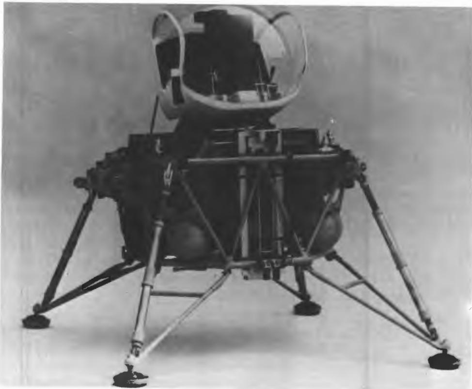
Above is a model of the prototype rocket-powered vehicle to be used in the lunar landing test facility at NASA's Langley Research Center. At the right is an engineering sketch of the way the facility would look when completed and in use.
