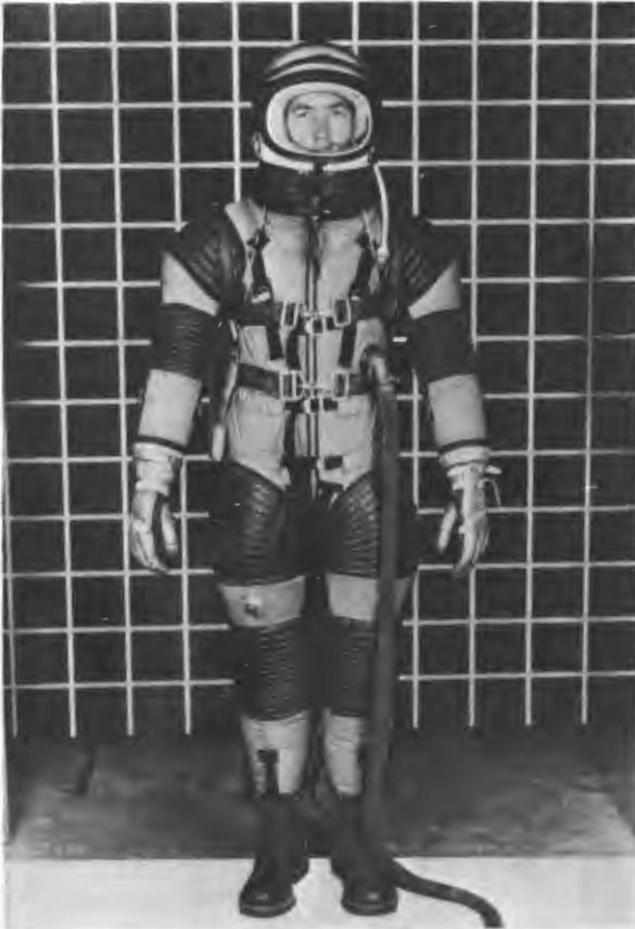
Many changes were made in space suits before the Apollo suit was finally developed in flight configuration. Joe Kosmo, Crew Systems Division, is shown on December 20, 1962, modeling a suit with constant volume joints constructed of restrained bellows.
