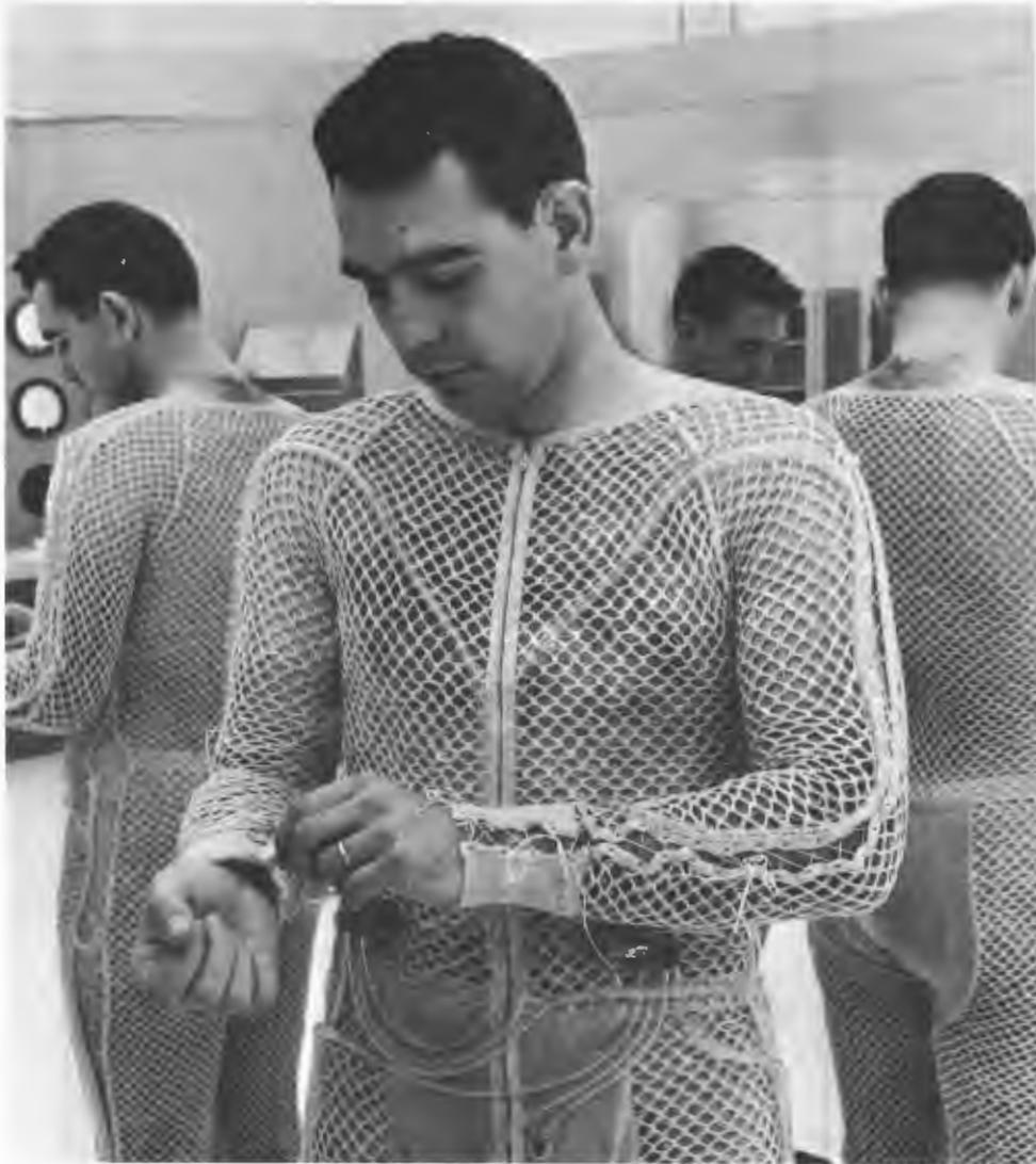
An experimental water-cooled garment, designed to cool space-suit-clad astronauts by water-filled tubes, was delivered to MSC's Crew Systems Division for evaluation. The garments were expected to allow astronauts to work harder and perform more tasks than originally expected.
