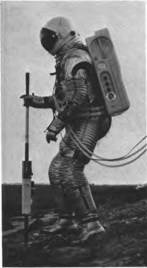
Randolph H. Hester of MSC's Crew Systems Division wore a pressurized space suit and a 13.6-kilogram (30-pound) backpack containing oxygen for coolant, pressurization, and breathing as he traversed a slope at MSC's "moonsite." During the test—part of a dress rehearsal for the crew performance, at Bend, Ore., August 24–28, 1964—Hester used a modified "Jacob's Staff," designed to help him keep his balance.
