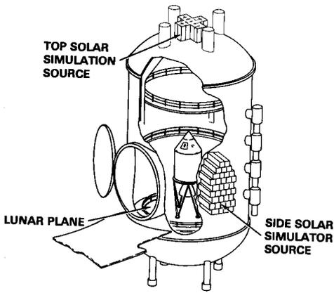
A cutaway view of the large space environment chamber in the Space Environment Simulation Laboratory at Manned Spacecraft Center shows how Apollo spacecraft components were tested at the extreme temperatures they would meet in space.
