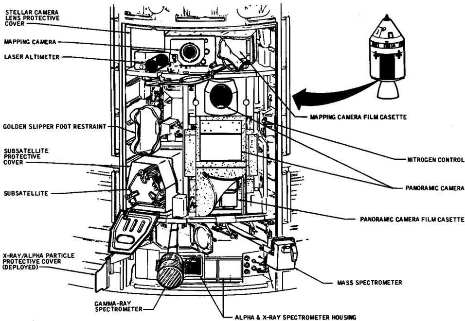
The SIM bay of the *Apollo 16* scientific instrument module housed sensors and experiments to gather data on the moon's atmosphere and surface, as well as a subsatellite to be launched in lunar orbit. Gamma ray and mass spectrometer sensors extended on a boom when in use.
