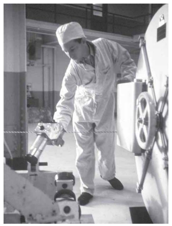
Image 80: A health-physics technician uses a hand-held "cutie pie" radiation detector to check equipment for contamination. These detectors allowed technicians to quickly monitor specific areas or equipment. They worked in conjunction with the permanent systems that constantly monitored radiation levels throughout the facility. (NASA C-2003-840)
