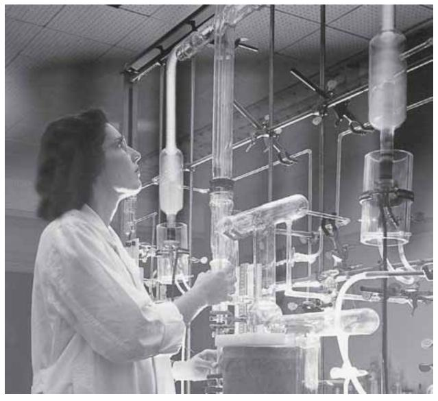
Image 30: One of the rare women physicists at NASA Lewis Research Center, working on an atomic laboratory experiment that pushed a gas at low pressure through a high-voltage discharge. (1957) (NASA C-1957-45726)
