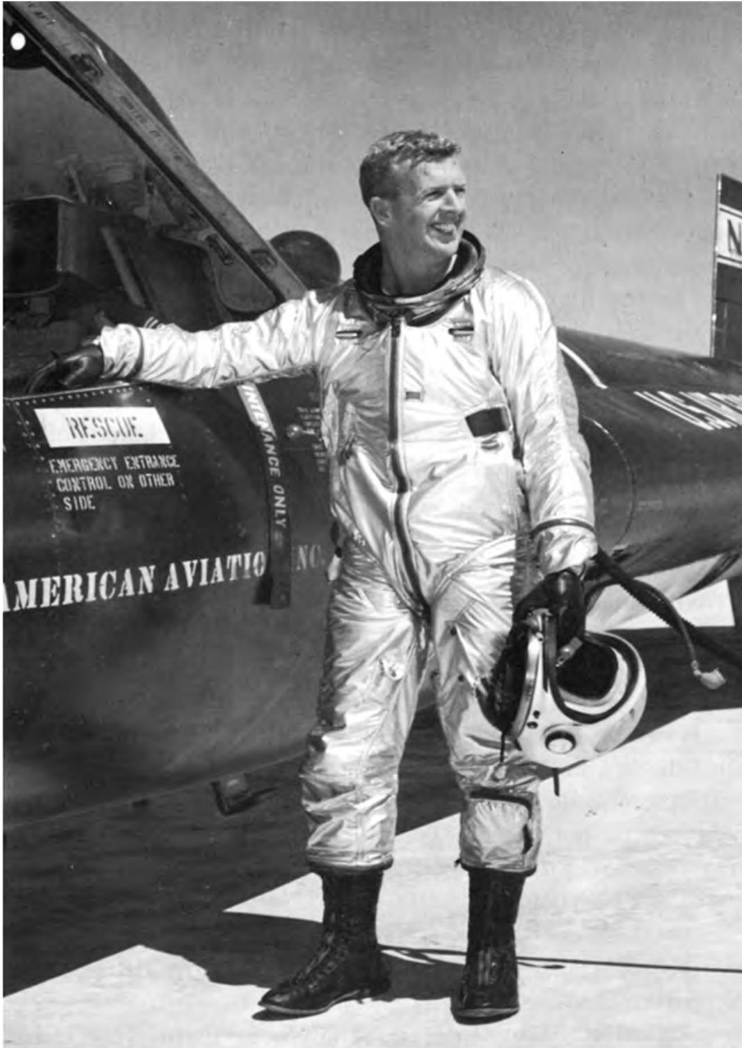
Chief Research Pilot Joseph A. Walker, of NASA's Flight Research Center, Edwards, Calif., stands beside an X-15 in full-pressure suit, the type that provides all X-15 pilots with livable atmosphere during flight. The dark tube attached to Walker leads to a portable unit that supplies each pressure-suit wearer with essential air-conditioning on the ground.
