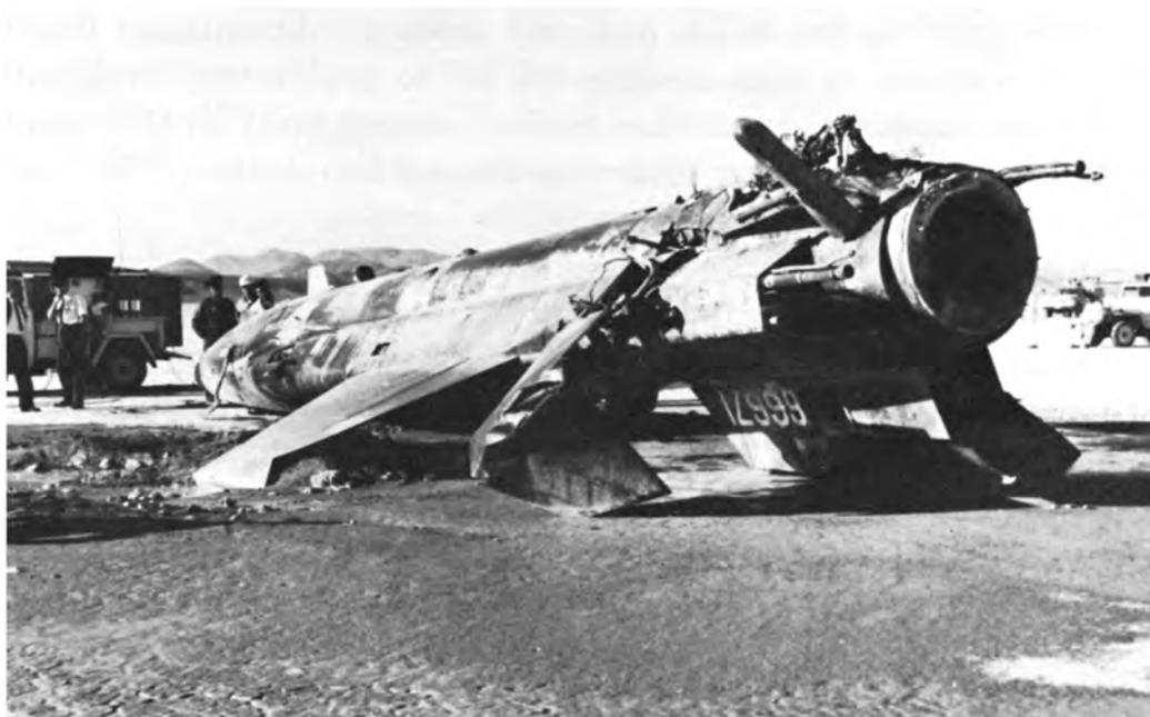
One such landing resulted in abnormally high loads because of a heavyweight condition from incomplete jettisoning of all unused propellants, and only partial cushioning of the nose impact by the nose-gear shock strut. When the nose wheels touched down, the fuselage buckled just aft of the cockpit, causing it to drag on the ground. Fortunately, the damage was easily repaired, and the airplane was back in the air within three months.
