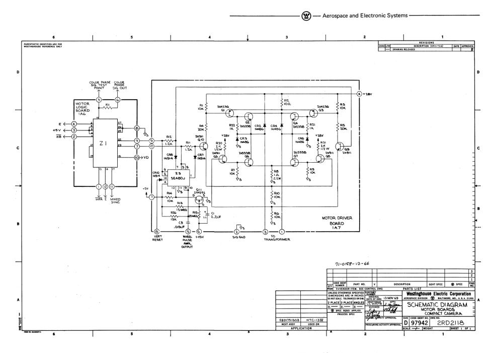
Figure 20. Motor Board Schematic
