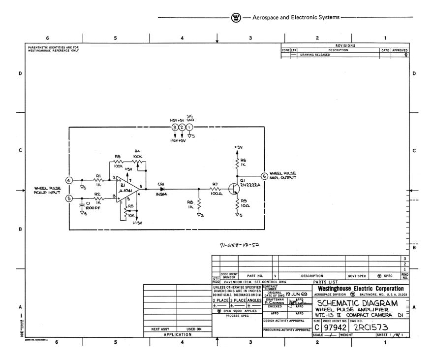
Figure 19. Wheel Pulse Amplifier Schematic
