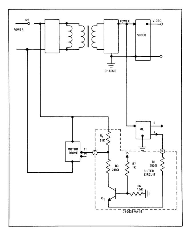
Figure 23. Filter Circuit Block Diagram
