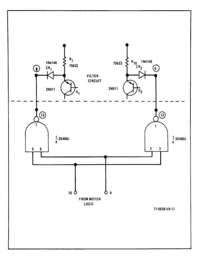
Figure 24. Fail Safe Circuit Schematic
