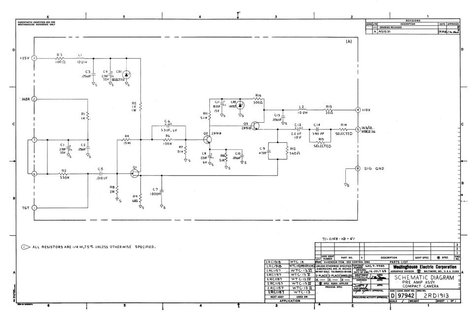
Figure 14. Preamplifier Schematic
