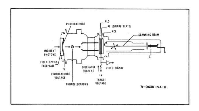
Figure 13. SEC Image Tube Layout
