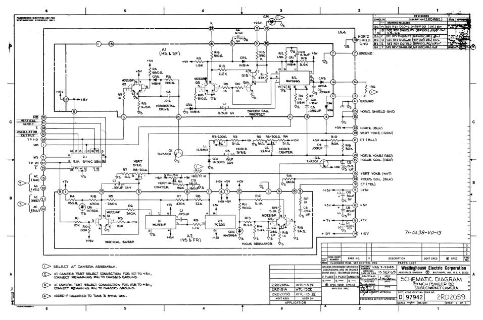
Figure 16. Sync/Sweep Board Schematic
