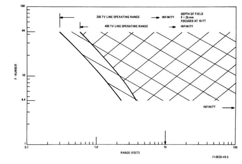
Figure 7B. Lens Depth of Field vs Zoom (25 mm)
