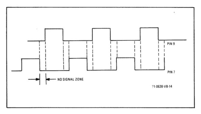
Figure 2b. Motor Input Signal Duty Cycle
