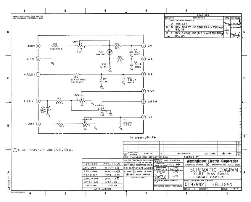
Figure 17. Tube Bias Board Schematic
