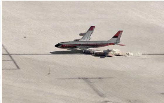
This image, taken in 1984, shows the Controlled Impact Demonstration, in which a Boeing 720 was flown remotely by a Dryden pilot onto Rogers Dry Lake. Embedded spikes tore open the wing tanks to see if a substance called Anti-Misting Kerosene (AMK) mixed in with the fuel would prevent the fuel from atomizing and catching fire. The huge ball of fire settled that question.
