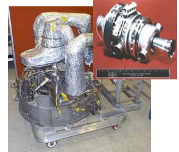
2 kW Brayton testbed
