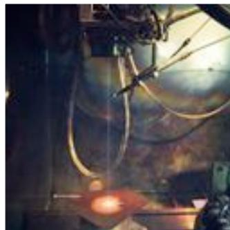
Electron beam freeform fabrication system: ground-based system (left); prototype schematic (right).
