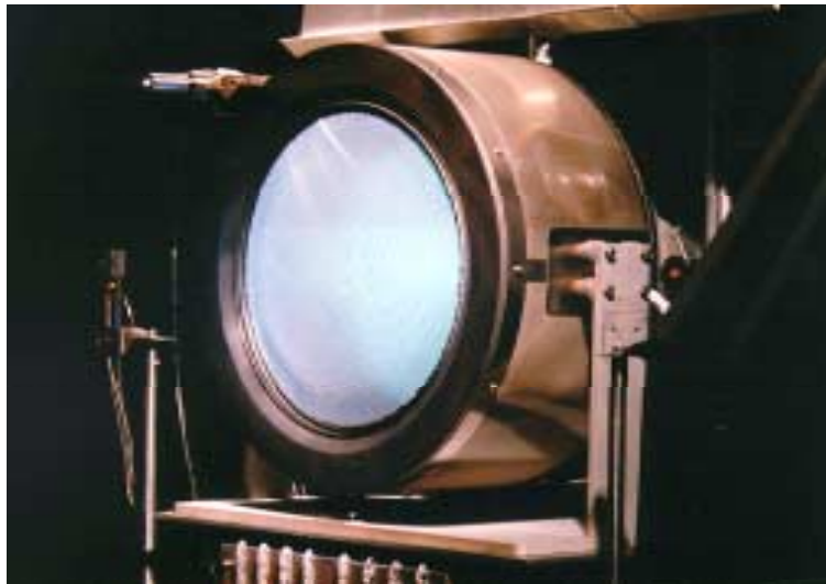
An 8200 Hour Test of an Ion Thruster (courtesy JPL).
