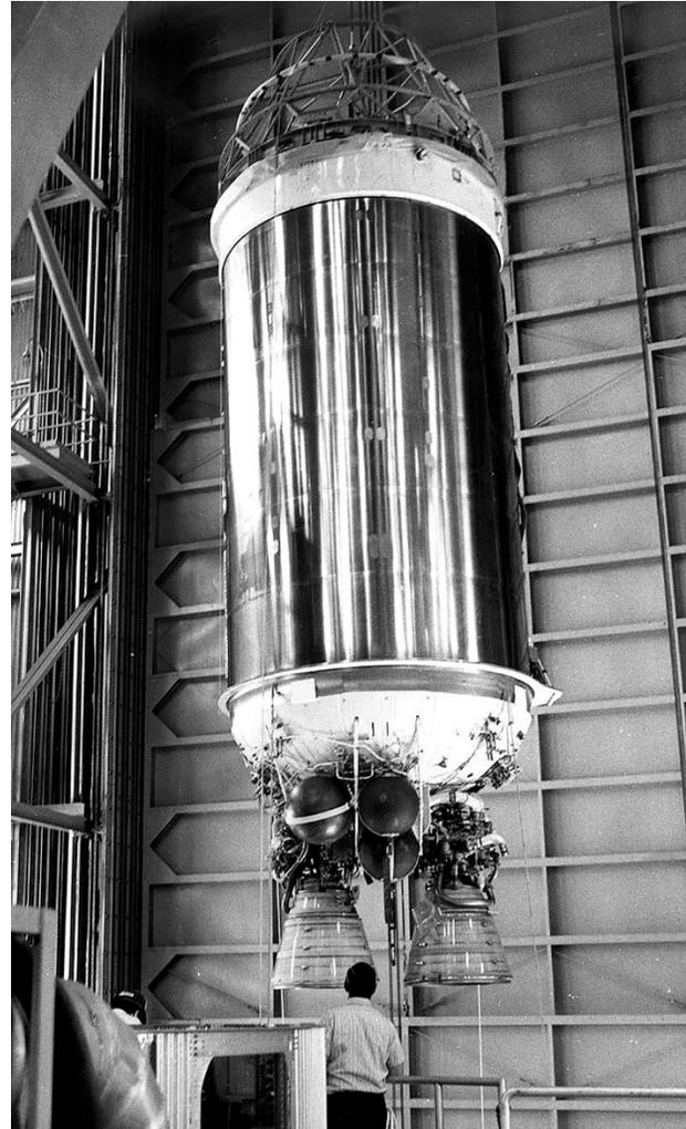
Image 162: A Centaur D-1T is prepared for mating with the Titan III booster in 1974 (NASA 101-KSC-74P-302).
