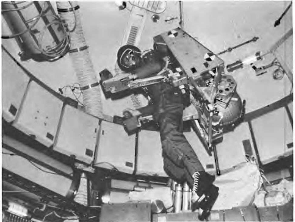
A *Skylab 3* onboard photo shows astronaut Jack R. Lousma as he flew the astronaut maneuvering unit in the forward dome of the space station while in Earth orbit.
