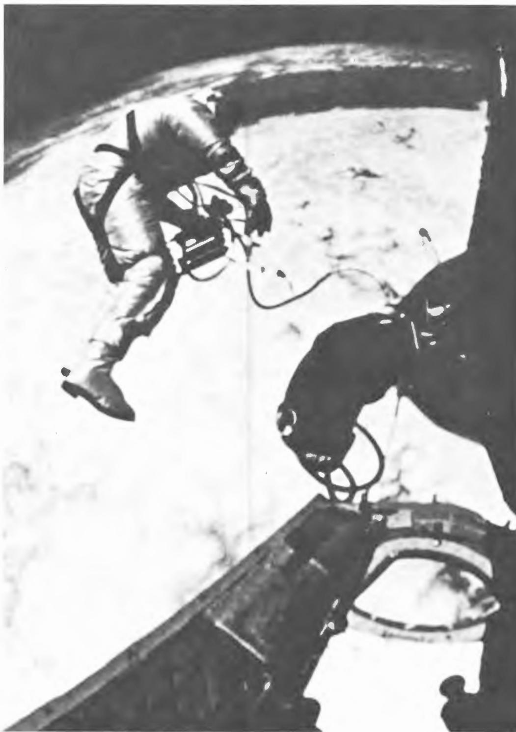
*Astronaut Edward H. White performs his spectacular space feat during the third orbit of the Gemini-Titan 4 flight. While floating, White is secured to the spacecraft by a 25-ft. umbilical line and a 23-ft. tether line, both wrapped together with gold tape to form one cord. White was the first American astronaut to egress his spacecraft while in orbit.*
