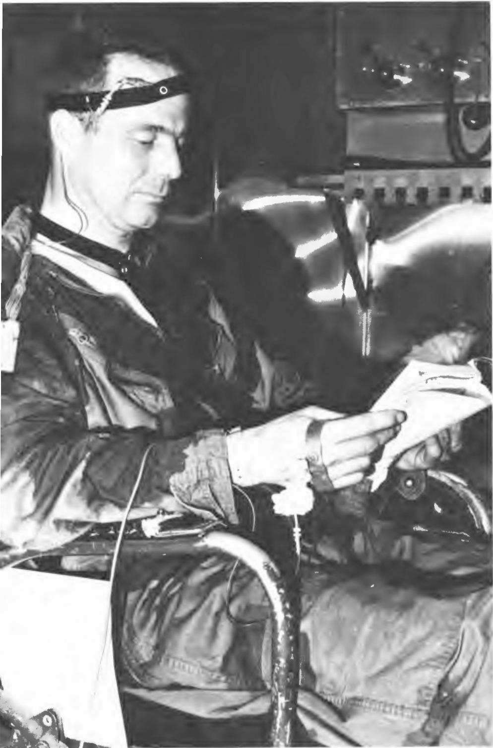
*Project Mercury astronaut candidates were put into a heat chamber for an extended period to measure their ability to function under the stress of heat. With the temperature at 130° F, Malcolm S. Carpenter spends the time reading.*
