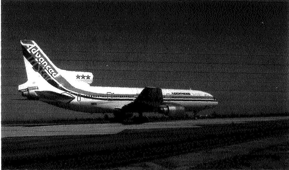
*Lockheed L-1011, showing its rear engine installation. (Lockheed)*
