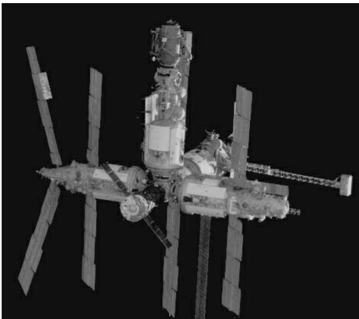
*Figure 10. Mir with new docking module (top, center of photo) installed on the Kristall module. The photo was taken by the departing Atlantis on STS-74. Spektr is shown at the left, Kvant 2 at the right.*
