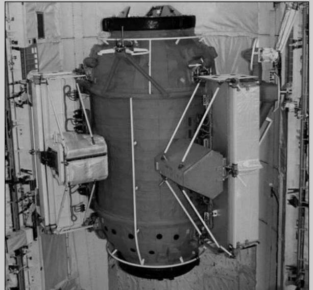
*Figure 9b. The Docking Module in Atlantis' payload bay before launch of the STS-74 mission.*
