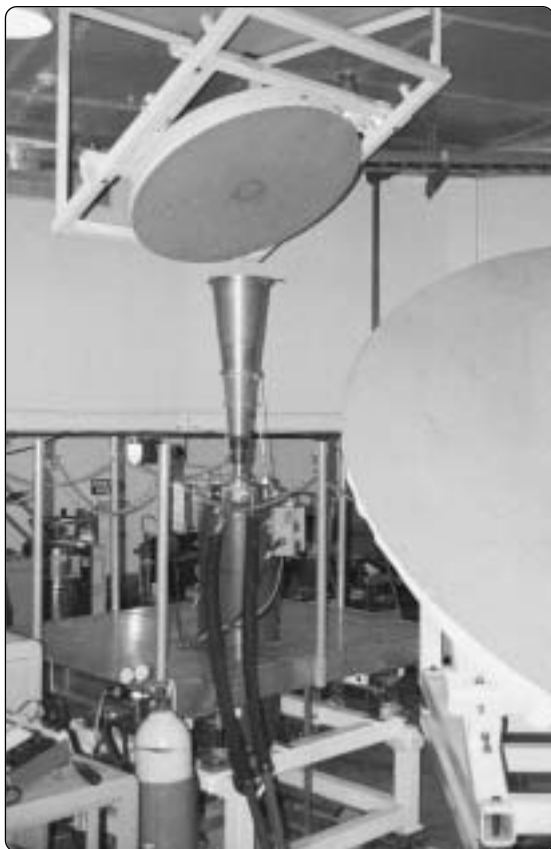
Figure 7-8. Ultra-low-noise amplifier (ULNA) at DSS 13.
