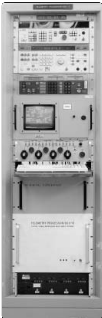
Figure 7-10. The Advanced Receiver (ARX) as used to track the Pioneer 10 spacecraft.
