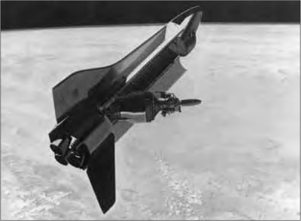
*Artist's rendering of Shuttle/Centaur preparing to launch payload. The bay doors are open, and the payload is about to be released by the Centaur Integrated Support Structure (CISS). (Glenn Research Center unprocessed photo)*
