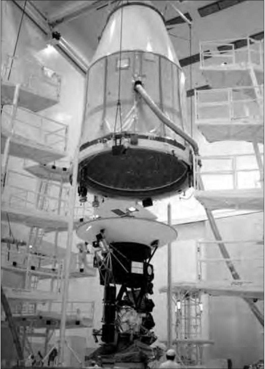
*The Voyager spacecraft as it is encapsulated within its protective shroud at the Spacecraft Assembly and Encapsulation Facility at Kennedy Space Center on 2 August 1977. It would later be mated with Titan-Centaur 7 for launch on 20 August 1977. (NASA KSC\_77P\_0201)*
