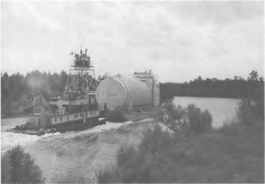
*The tugboat Apollo heads down river to New Orleans for another load of liquid hydrogen to support Space Shuttle Main Engine testing. (SSC-78-447-27)*
