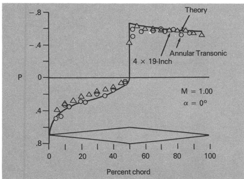
FIGURE 6.—Guderley theory for Mach 1 compared with Langley transonic tunnel data.
