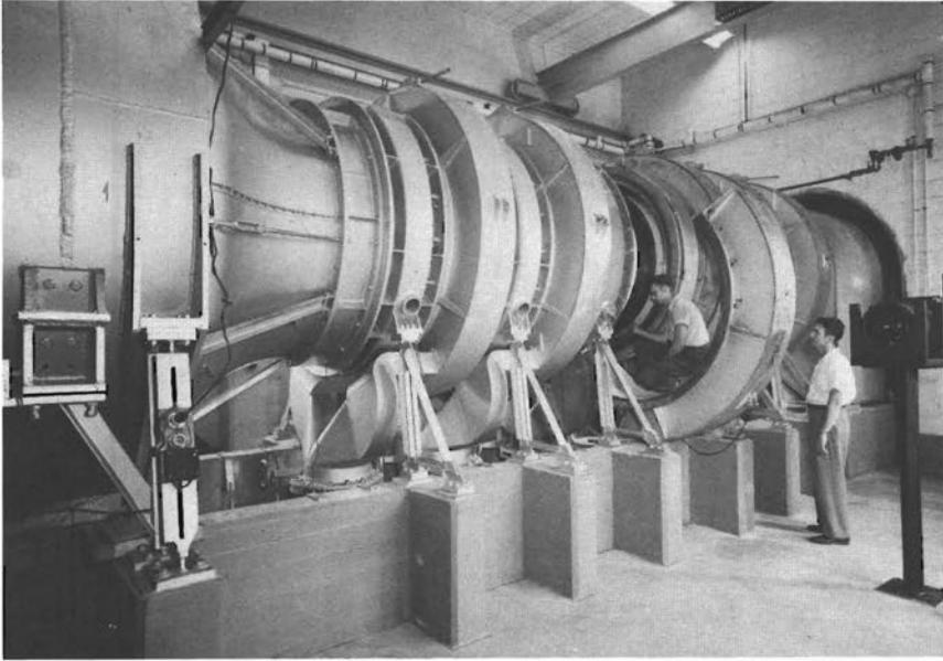
FIGURE 20.—*The Annular Transonic Tunnel, opened at the rotor section. R. Turner, left, and L. W. Habel.*
