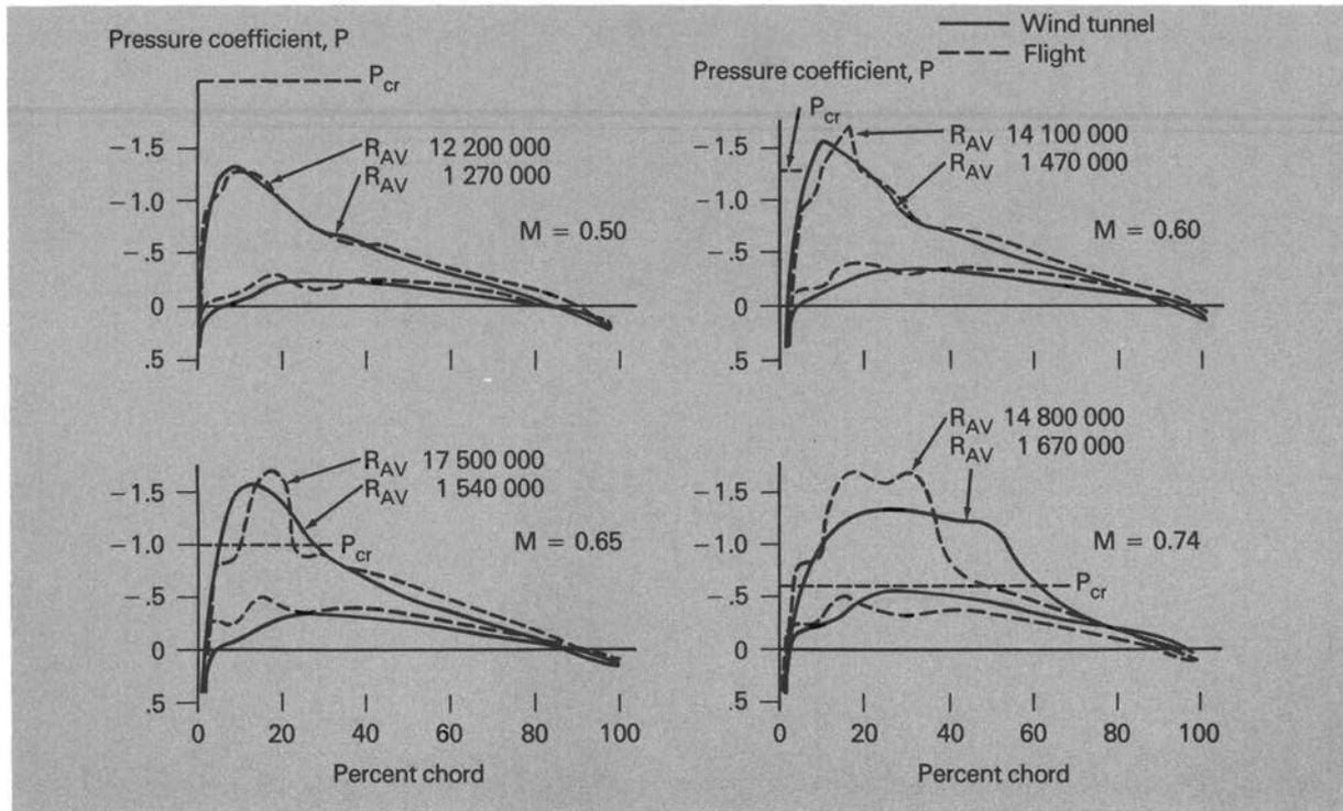
FIGURE 21.—Comparison of flight and wind tunnel pressure-distribution measurements for  $C_n = 0.4$ ; airplane wing, NACA 230-series section  $14\frac{1}{3}$  percent thick; wind tunnel model, NACA 23015 section.
