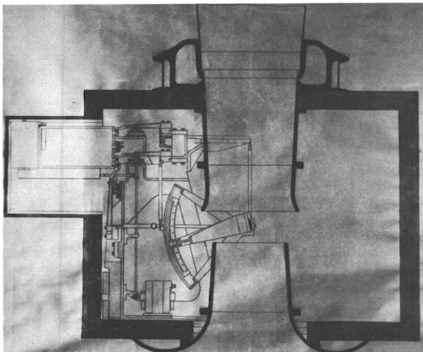
FIGURE 11.—*The Langley 11-Inch High-Speed Tunnel with the open throat developed in 1930.*
