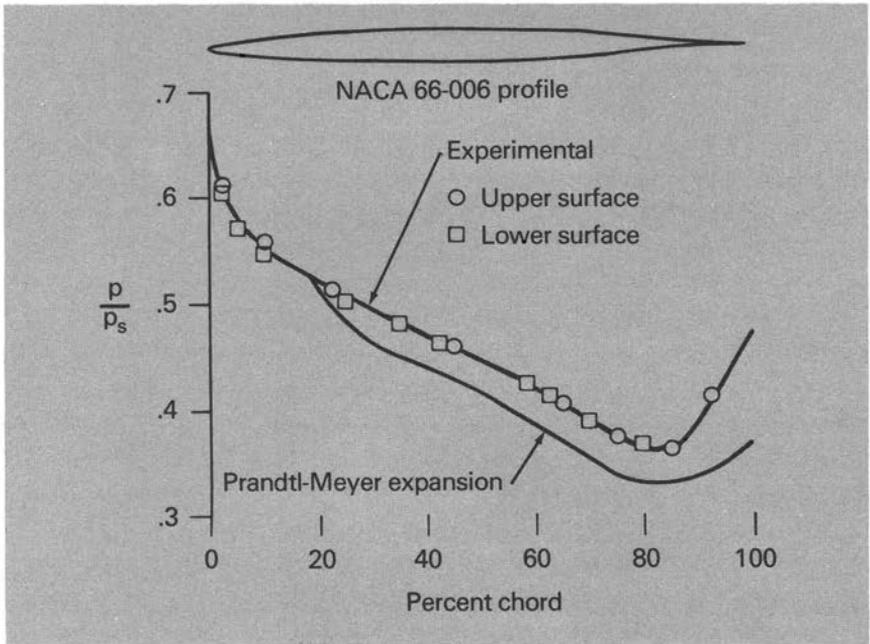
FIGURE 7.—Pressure distribution obtained in the Langley Annular Transonic Tunnel at Mach 1. NACA 66-006 airfoil at zero angle of attack.
