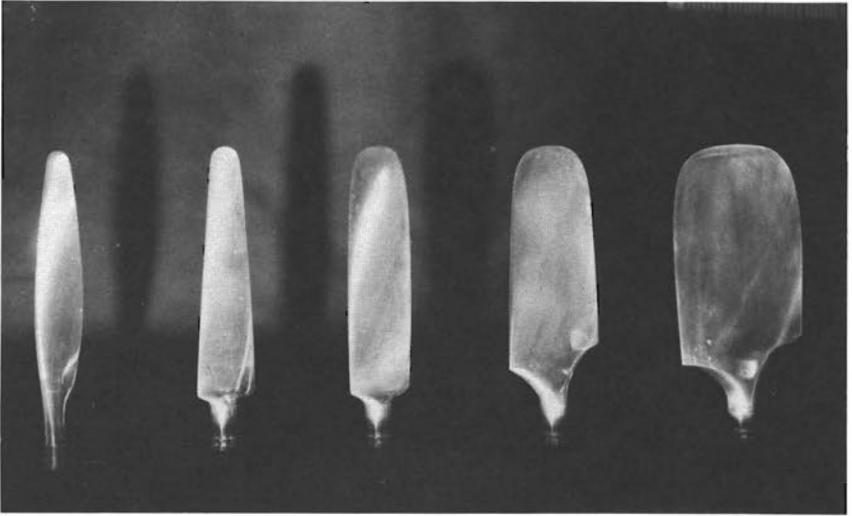
FIGURE 29.—Blade shapes tested in the Emergency Propeller Program in the 8-Foot High-Speed Tunnel.
