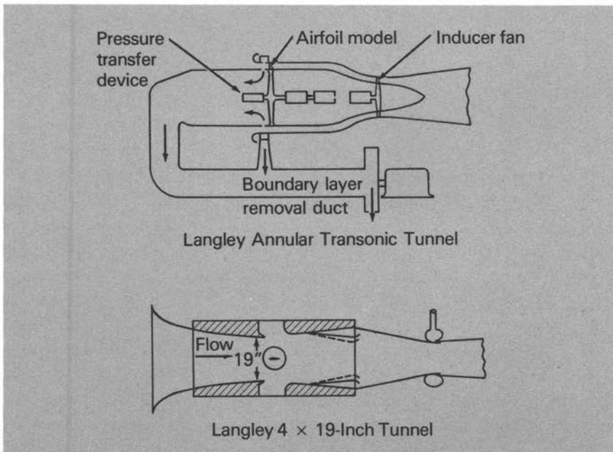
FIGURE 18.—Schematic drawings of the Annular Transonic and the 4 x 19-Inch tunnels.
