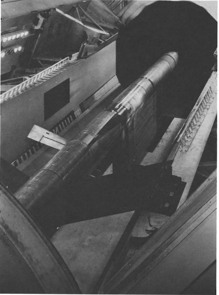
FIGURE 35.—*The 6000-hp Propeller Dynamometer installed in the re-powered slotted 16-Foot High-Speed Tunnel.*
