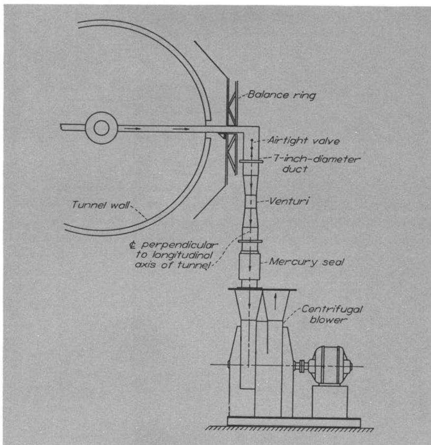
FIGURE 38.—Blower installation in 8-Foot High-Speed Tunnel for investigation of high-speed air inlet and outlet openings, and the principal shapes tested.
