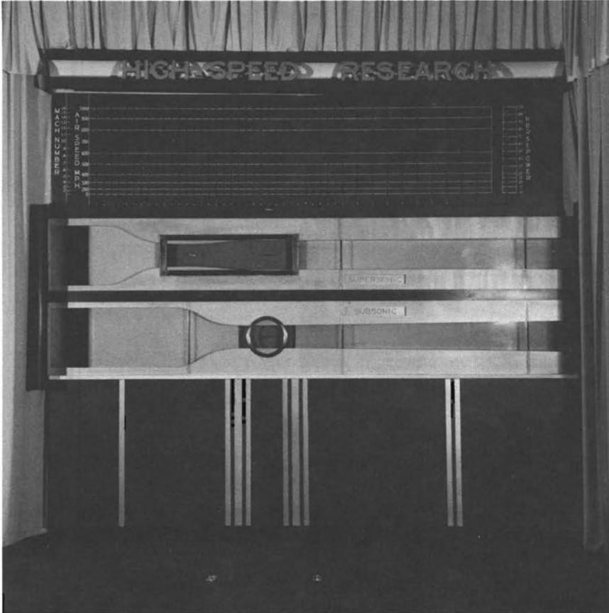
FIGURE 17.—Small tunnels used to demonstrate choking, supersonic nozzles, power requirements, and transonic and supersonic airfoil flows, 1946.
