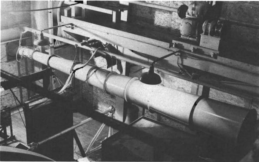
FIGURE 23.—"Parasite" tunnel used to test the first successful slotted throat. The 12-inch diameter test section is at extreme left. Tunnel operates by suction of outside air into the test chamber of the 16-Foot High-Speed Tunnel.
