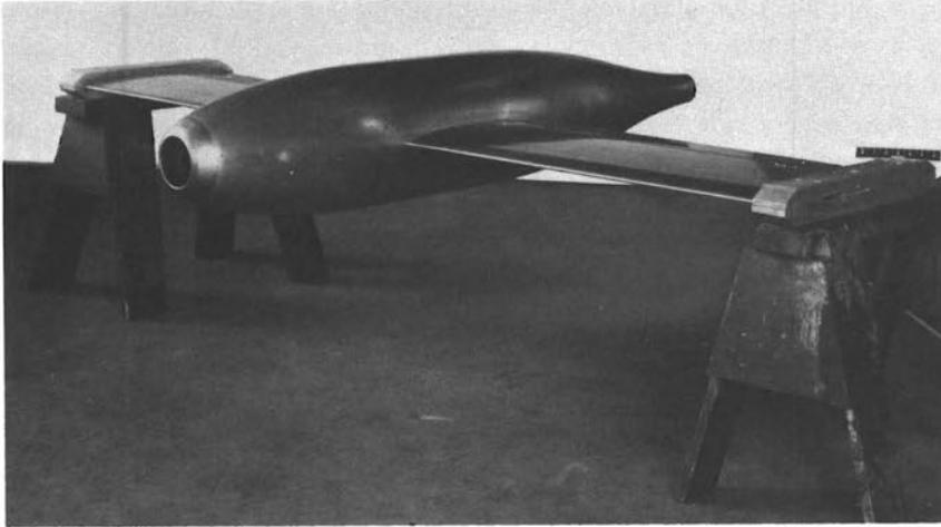
FIGURE 42.—“Heat model” used in the first NACA investigation of a propulsive-duct (ramjet) system in the 8-Foot High-Speed Tunnel in February and March 1941. Model incorporated a 160-kw heater. Nose B and cusped outlet from ref. 179.
