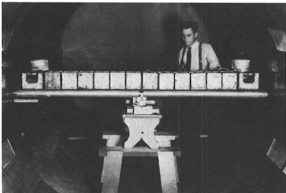
FIGURE 2.—*Typical airfoil in the original 8-Foot High-Speed Tunnel, weighted to determine deflection corrections. J. V. Becker in photo, 1937.*
