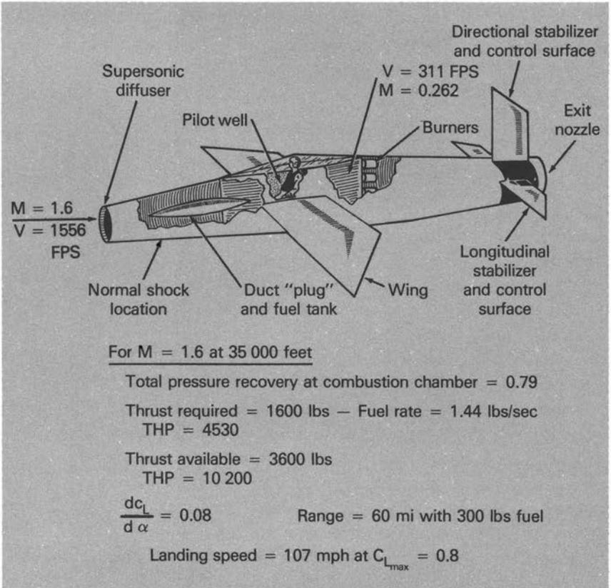
FIGURE 22.—*Ramjet-powered configuration analyzed by Ellis and Brown, 1944–1945. From a Langley Conference chart.*
