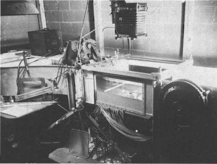
FIGURE 12.—*Water channel used by the 8-foot tunnel group to investigate tunnel choking phenomena by means of the hydraulic analogy.*
