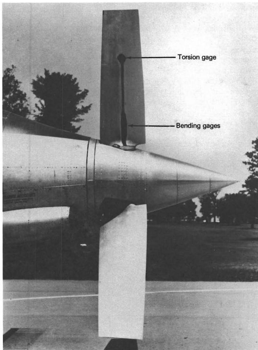
FIGURE 36.—Supersonic propeller (feathered) driven by T-38 turboprop engine mounted on XF-88 propeller research airplane.
