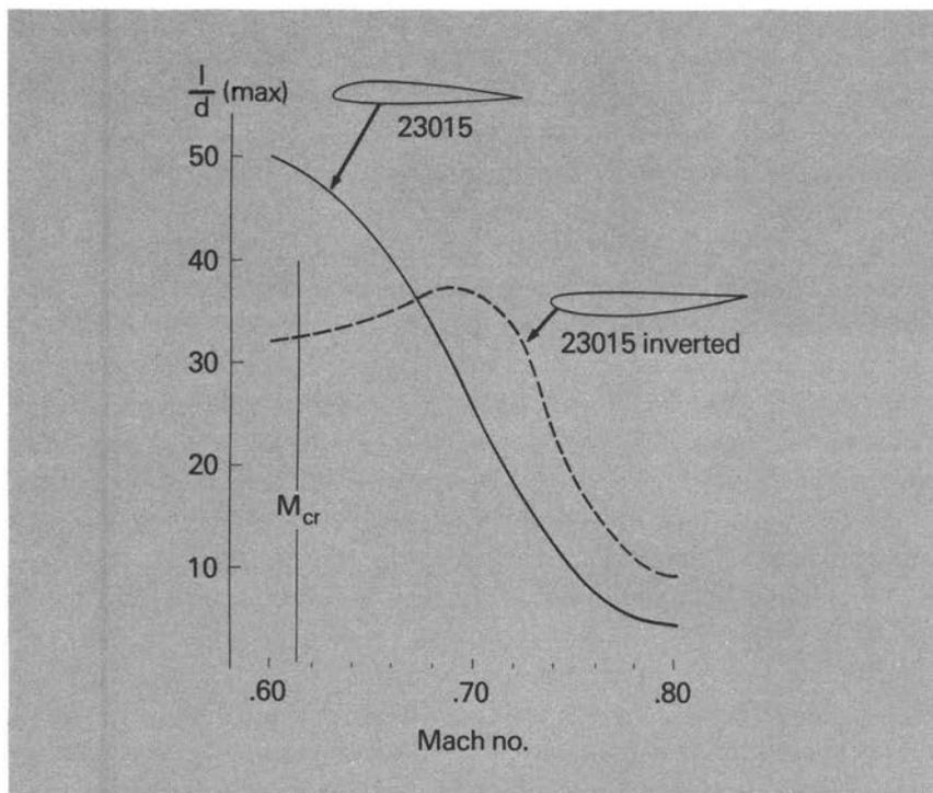
FIGURE 8.—Improvement in supercritical lift-drag ratio ( $l/d$ ) with negative camber. Ames data, 1945.
