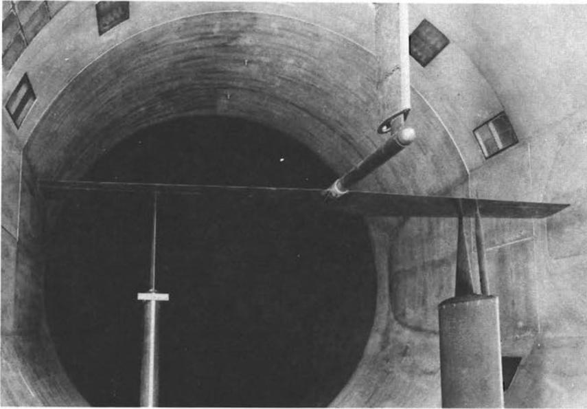
FIGURE 13.—*Typical strut support system used prior to 1944 in the 16-Foot High-Speed Tunnel. Choking speed was about Mach 0.8.*
