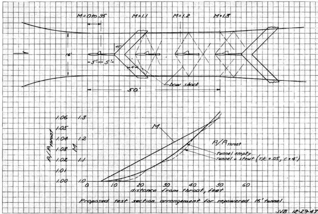
FIGURE 25.—Fixed-geometry nozzle with variable model position for transonic testing up to Mach 0.95 and from 1.10 to 1.30. This was one of several schemes put forward in the 1946–1948 time period as alternatives to the slotted throat.
