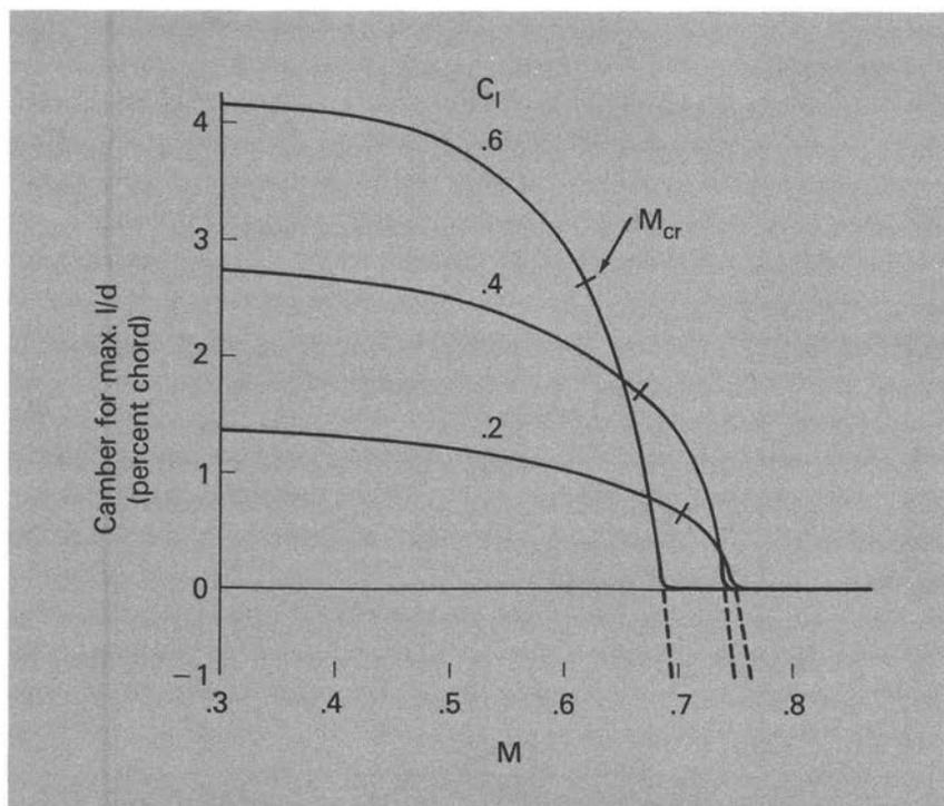
FIGURE 9.—Effect of Mach number on camber for best lift-drag ratio. 12-percent-thick airfoils.
