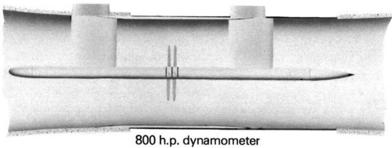
FIGURE 14.—Support systems developed by Langley which do not cause a decrease in choking Mach number. From a 1946 Conference chart.
