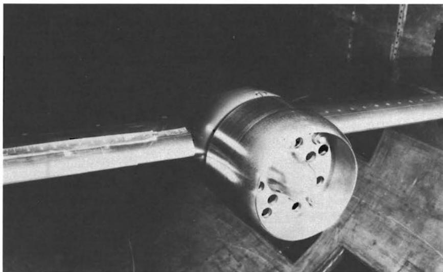
FIGURE 37.—*High-speed cowling test setup in the 8-Foot High-Speed Tunnel, 1937.*
