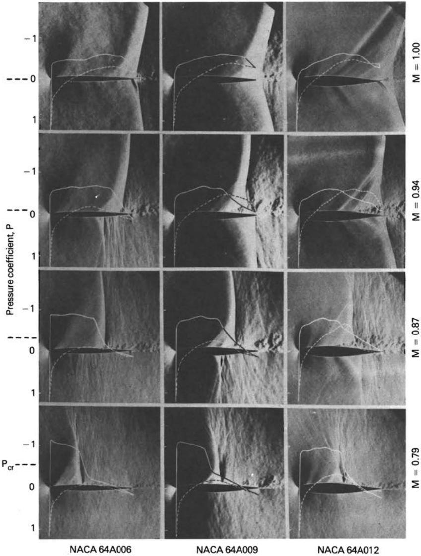
FIGURE 4.—*Transonic flows and pressure distributions, Mach 0.79 to 1.00. Angle of attack, 3.2 deg. From the 4 x 19-Inch Semi-Open High-Speed Tunnel, 1949.*
