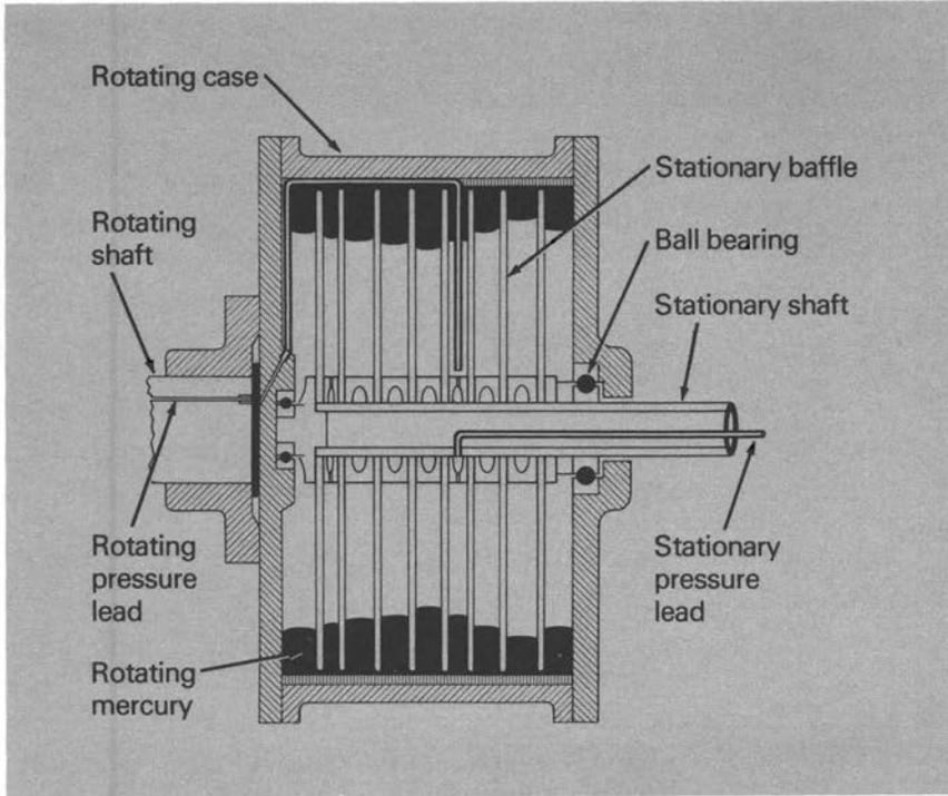
FIGURE 19.—Section through axis of rotation of the pressure-transfer device of B. W. Corson, Jr.
