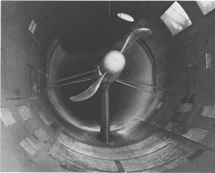
FIGURE 33.—*The swept-blade propeller tested on the 2000-hp dynamometer.*
