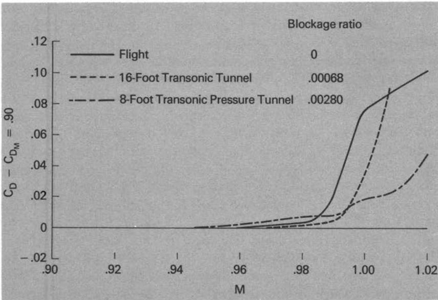
FIGURE 24.—Comparison of flight (drop tests) and slotted-tunnel drag data showing discrepancies at Mach numbers above 0.98, 1973 data.
