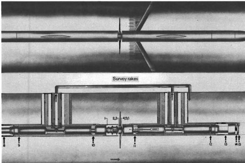
FIGURE 34.—*The 800-hp Propeller Dynamometer used in the repowered 8-Foot High-Speed Tunnel.*
