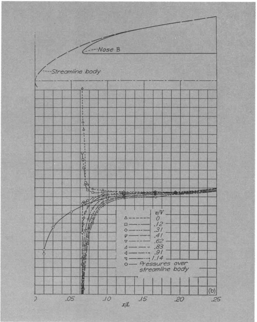
FIGURE 39.—Typical drag, transition, and pressure data from inlet-outlet investigation.
