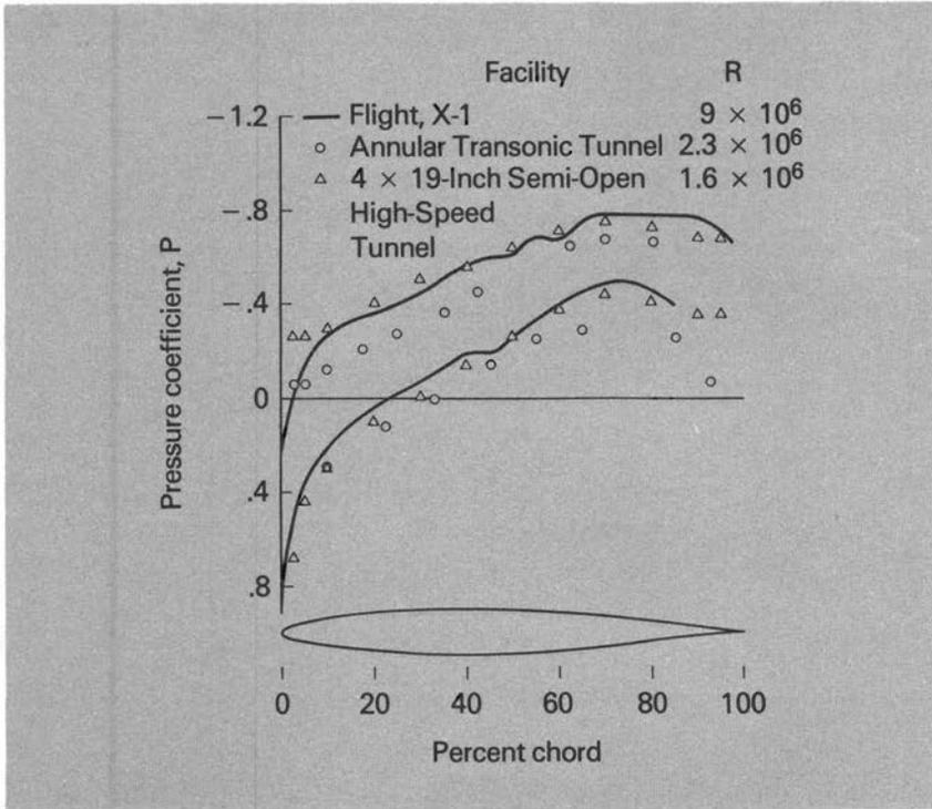
FIGURE 5.—The X-1 pressure distributions compared with those of the Annular Transonic and the 4 x 19-Inch tunnels. Mach 1.0, NACA 65-110 airfoil,  $c_n = 0.41$ .
