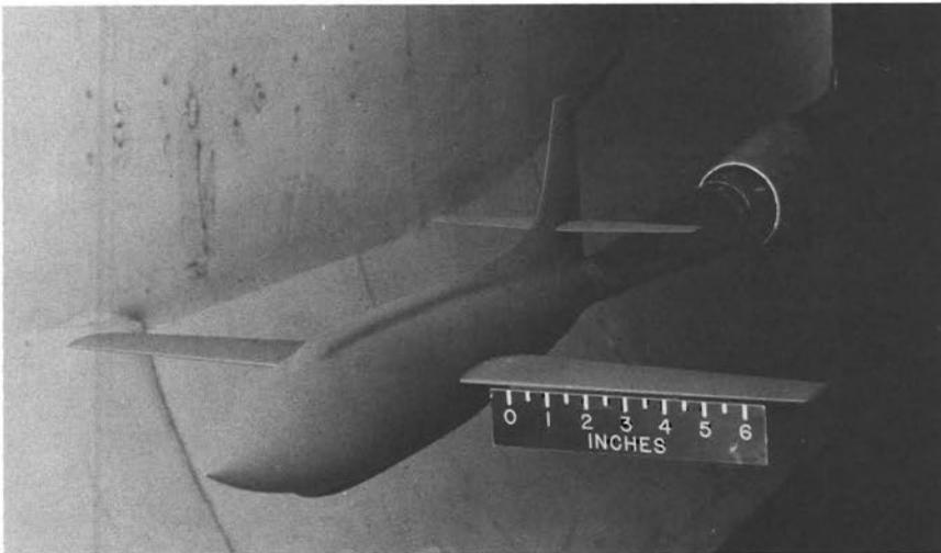
FIGURE 16.—Sting-supported model of the X-1 in the repowered 8-Foot High-Speed Tunnel, 1946.
