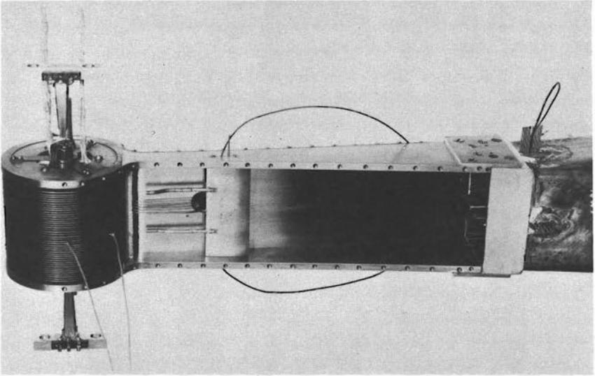
FIGURE 41.—*Electrically heated finned-cylinder model used by 8-foot tunnel group to investigate cooling-airflow relationships at high speeds.*
