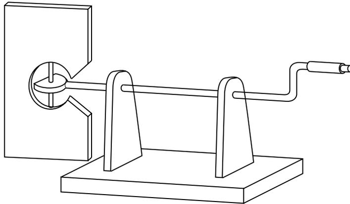
**(b) Rotation about axis of maximum inertia. When rotation is started with the plate in this position, it remains in this orientation during the rotation.**
