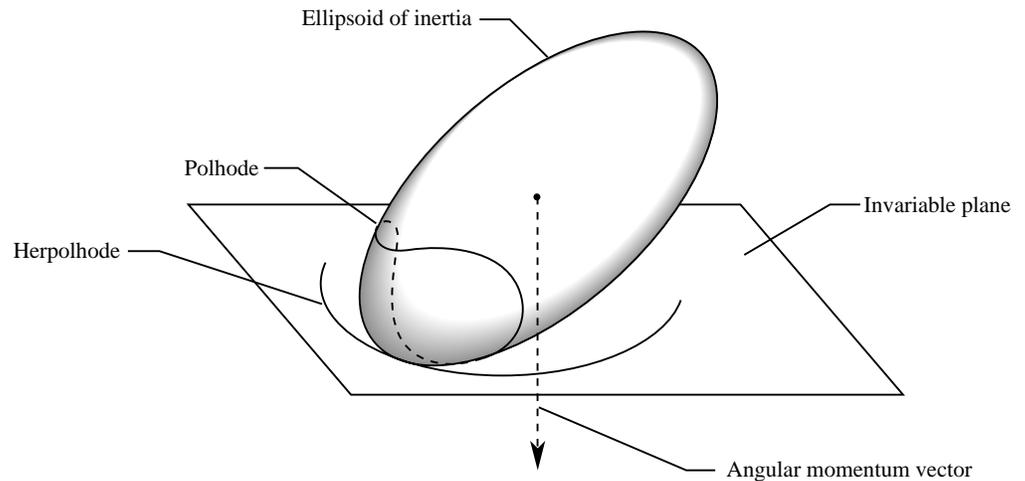
body may be described by the moments of inertia about three mutually perpendicular axes, with their origin at the center of gravity, called the principal axes of inertia. These values of moments of inertia, represented as vectors  $I_X$ ,  $I_Y$ , and  $I_Z$  along the three principal axes, can be used to determine the axes of an ellipsoid, called the ellipsoid of inertia. The shape of the ellipsoid is determined by the mathematical formula for an ellipsoid:
