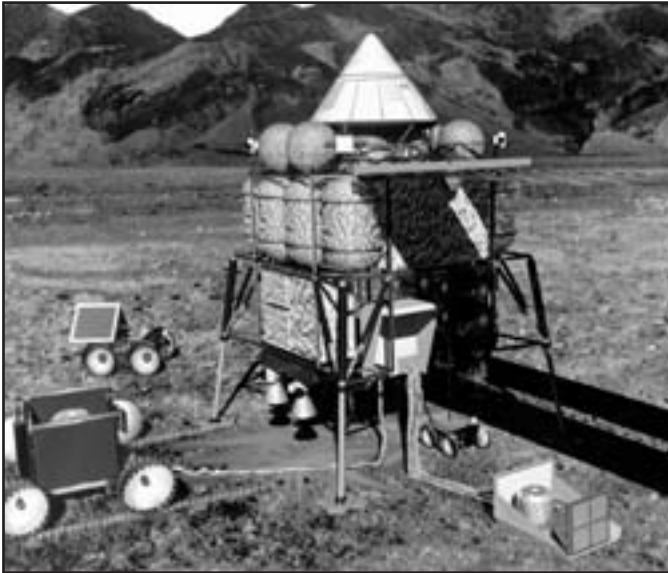
Figure 23—NASA's 1993 Mars mission plan: after landing on Mars, the automated propellant factory manufactures liquid methane and liquid oxygen propellants for the conical Mars Ascent Vehicle it carries on top. (NASA Photo S93-50643)
