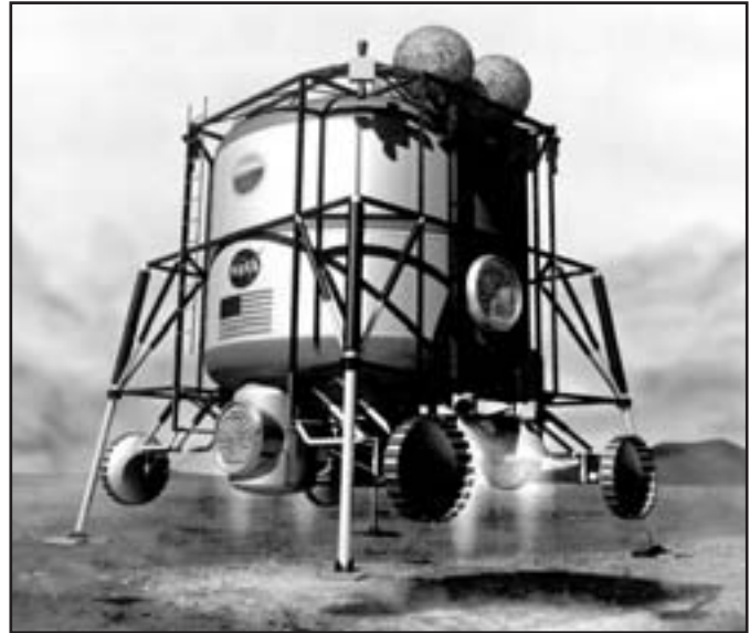
Figure 24—The crew Habitat lands near the propellant factory with empty propellant tanks. Note wheels for moving the Habitat on the martian surface. (NASA Photo S93-050645)
