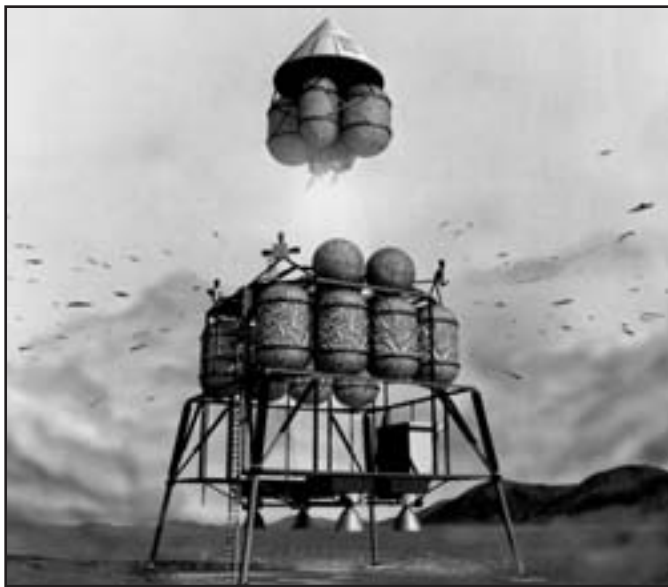
Figure 26—Using the propellant factory as a launch pad, the Mars Ascent Vehicle blasts off burning propellants made from terrestrial hydrogen and Martian atmospheric carbon dioxide. (NASA Photo S93-050644)
