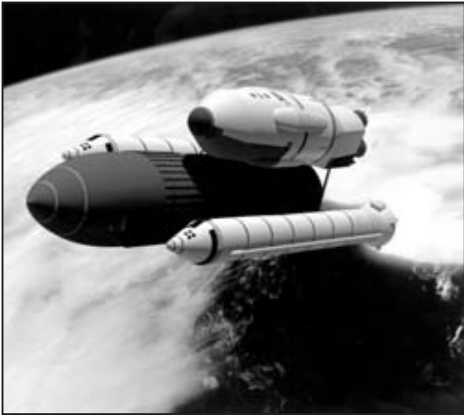
Figure 28—NASA's 1997 Mars plan proposed to reduce weight by using an aerobrake integrated with the spacecraft hull and nuclear rockets. These steps would help eliminate need for a heavy-lift rocket, permitting a cheaper Shuttle-derived launch system. (NASA Photo S97-07844)
