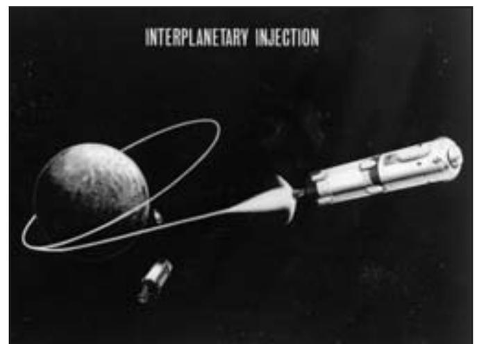
Figure 9—Three modified Apollo S-IVB stages burn one after the other to launch the 1967 Planetary Joint Action Group Mars flyby spacecraft out of Earth orbit. (NASA Photo S-67-5998)
