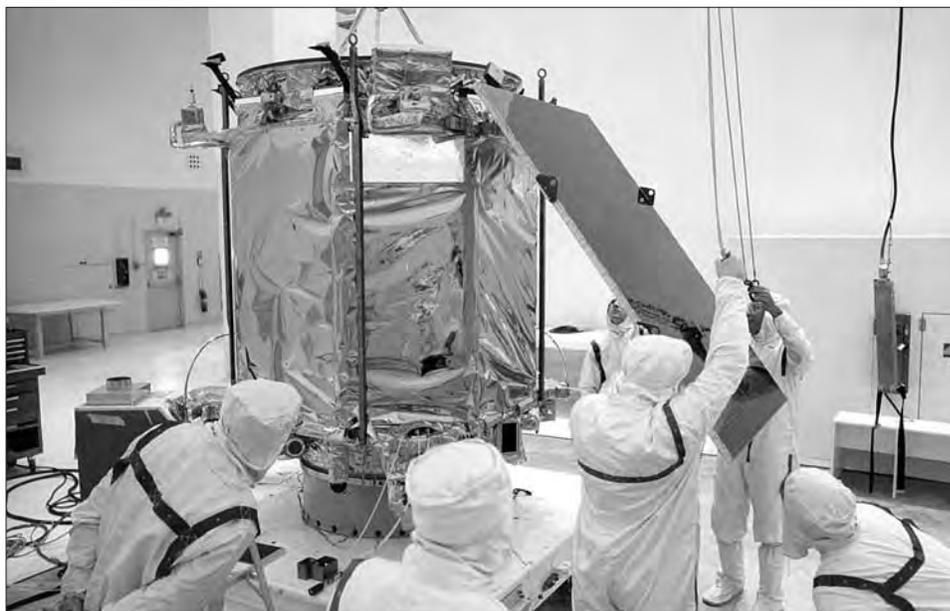
In the photograph above, workers in the Spacecraft Assembly and Encapsulation Facility-2 at Kennedy Space Center attach the solar array panels to the Near-Earth Asteroid Rendezvous (NEAR) spacecraft. After the fueling and battery installation, the spacecraft launched on a Delta II expendable launch vehicle provided by McDonnell Douglas. After a one-day delay, the NEAR spacecraft lifted off from Cape Canaveral Air Station at 3:43 p.m. EST, 17 February 1996.
