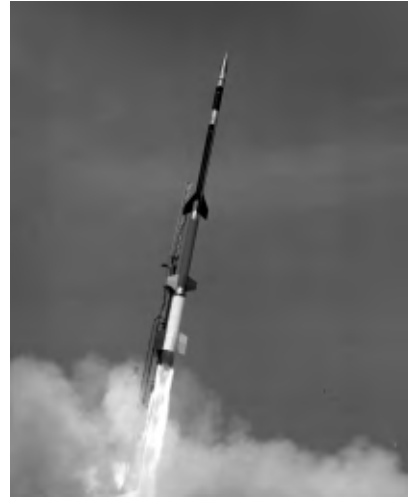
A Black Brant XII sounding rocket takes flight from Wallops Island. The four-stage rocket can fly to altitudes higher than 800 miles.
