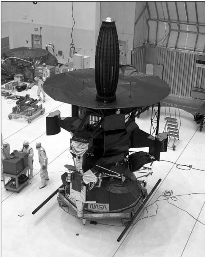
In the Vertical Processing Facility (VPF), the spacecraft Galileo is prepared for mating with the Inertial Upper Stage booster. Galileo was launched aboard the orbiter *Atlantis* on Space Shuttle mission STS-34, 12 October 1989, and sent to the planet Jupiter on a journey that took more than six years to complete. (GRIN Image GPN-2000-000672)
