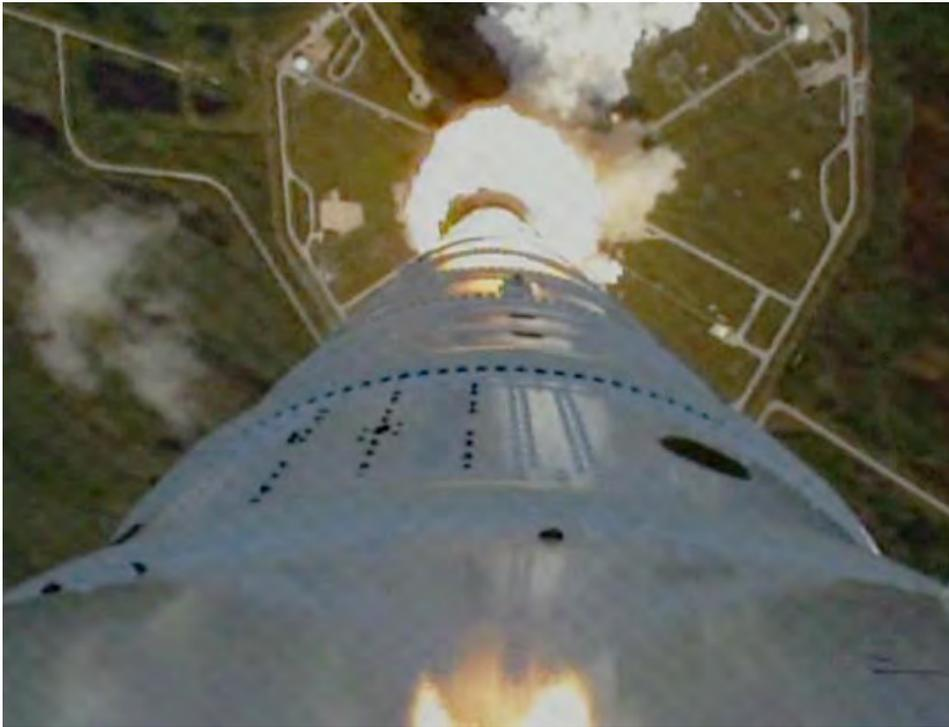
The Ares I-X test flight lasted about six minutes from its launch until splash down of the rocket's booster stage nearly 150 miles down range. This shot was taken from the rocket looking back at the launch pad. The roll control motors were used to control the vehicle during flight.
