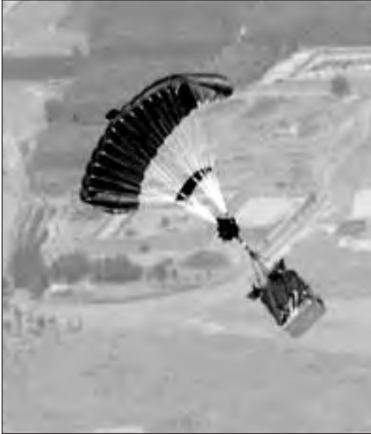
Onyx autonomously guided parachute system using GPS navigation.
